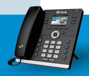
Display a colori 2.8" retroilluminato 320x240 px Due porte Gigabit, PoE 3 VoIP accounts, 8 soft keys SIP (RFC3261)/SIP v1 (RFC2543), v2 (RFC3261) Auto provisioning via HTTP/HTTPS FTP/TFTP 802.1X/OpenVPN/DHCP/Vlan/Qos/LLDP TLS/UDP/TCP, RTP/RTCP/ZRTP/SRTP HD Voice: Codec, Vivavoce, Microtelefono EHS certificato con cuffie Jabra, Sennheiser, Plantronics
